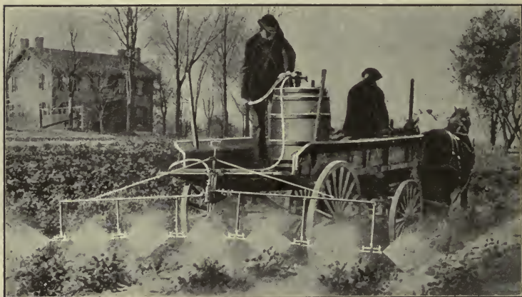
39. A POTATO SPRAYER FOR BUGS AND BLIGHTS
